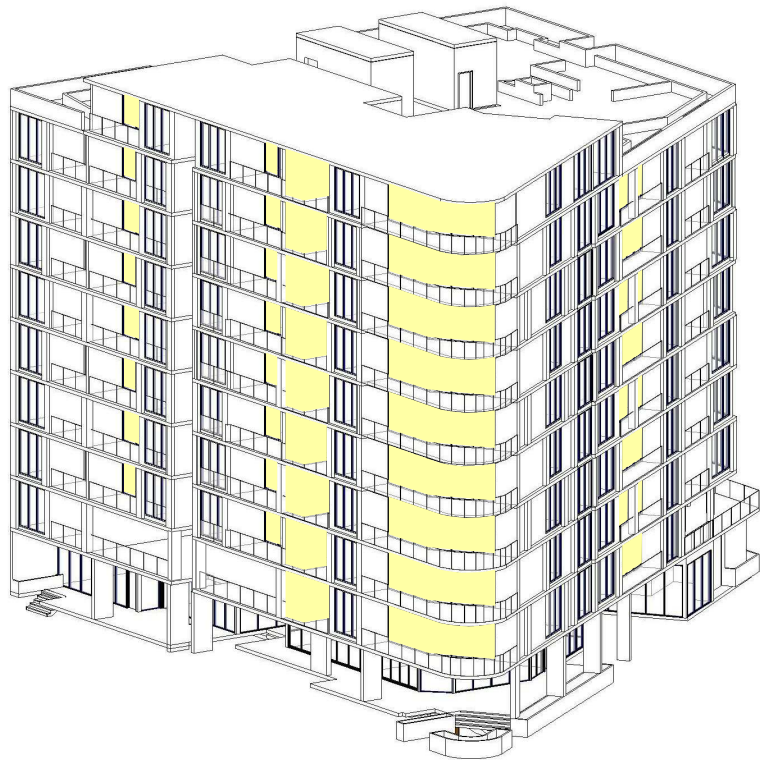
DIRECT SUNLIGHT ANALYSIS - MID-WINTER - 9AM AZIMUTH: 42°34'30" ALTITUDE: 18°58'55"
